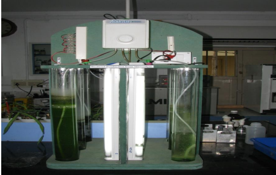
Fig.7. Photobioreactor for algae cultivation (30L capacity)
